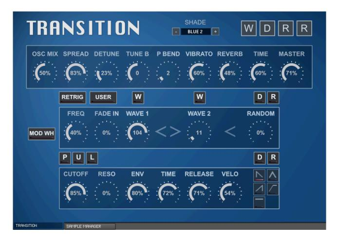
Transition & digiTs are based around a simple idea of cross fading between 2 waveforms or alternatively the Mod Wheel can be used for a manual fade position.
