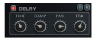
The Delay is a Send Effect which means that the signal is sent to it via the dedicated Sequencer which controls the amount sent. The overall Volume of the output is controlled by the FX knob in the Master section.
