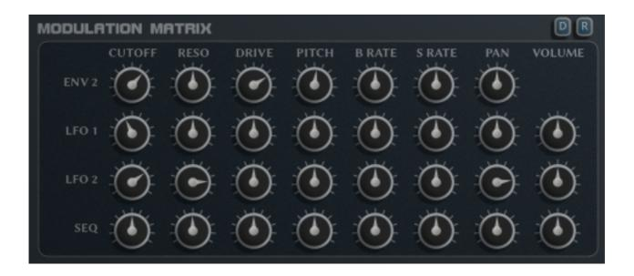
The Modulation Matrix is used to assign Modulator Amounts to Destinations. There are 4 Modulators available; Envelope 2, LFO 1, LFO 2 and the Sequencer. Centred Knobs mean no effect, left of centre has a negative impact and right of centre has a positive impact.
