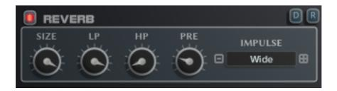
The Reverb uses Impulse Responses to generate the Reverb. It is a Send Effect which means that the signal is sent to it via the dedicated Sequencer which controls the amount sent. The overall Volume of the output is controlled by the FX knob in the Master section.
